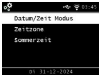
The device is set at the factory so that the time is set automatically. If the device is connected to the Internet via the network, the time and date are synchronised automatically. You therefore do not need to set the time manually. Select here how the radio should synchronise the time.
