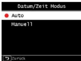
The device is set at the factory so that the time is set automatically. If the device is connected to the Internet via the network, the time and date are synchronised automatically. You therefore do not need to set the time manually. You can change these settings at any time in the main menu under System.
